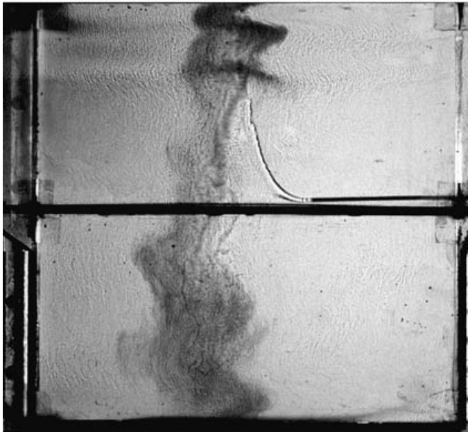
FIGURE 2. Shadowgraph pictures of two contrasting experiments, both of which developed vigorous convection upwards and downwards. (a) A salt plume, denser than the sugar solution into which it flowed by 6 parts in 10^4 , 100 min after the input started at 5 \text{ ml min}^{-1} . Later measurements showed that nearly equal amounts of salt were transported up and down. (b) A sugar plume (lighter by 8 parts in 10^4 ), flowing into salt solution at 5 \text{ ml min}^{-1} . Photo taken at 80 min after the start and 2 min after a dye streak was added near the centre. In this case, substantially more sugar was transported down than up, which is not obvious from the visual observations.
